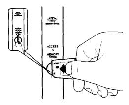
Be sure to insert the Memory Stick in the correct direction. If the Memory Stick is forced in the wrong way, it may become damaged.
